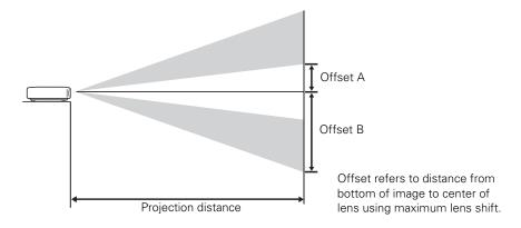
If you place the projector off to the side, aim it straight ahead (rather than at the center of the screen), then use the horizontal lens shift dial to center the image on the screen.
